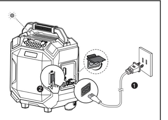
Charge the speaker until all four charging indicators light up, indicating that the battery is fully charged.
