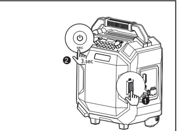
Make sure the power switch is in **I** position, then hold **SRC** to switch on.
