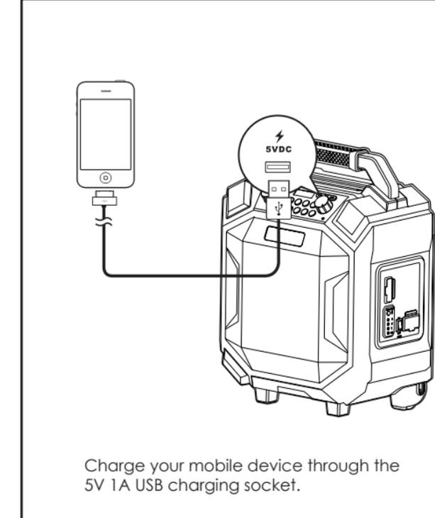
Charge your mobile device through the 5V 1A USB charging socket.
